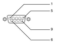
2) Connector on the external equipment side: Serial port (RS-232C) connector
